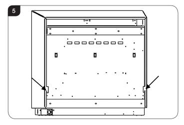
Let the legs spring back once over the top bar to engaged with the lower bar.
