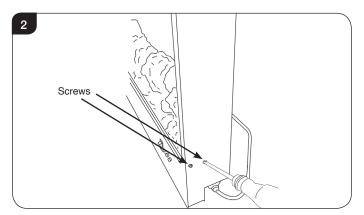
4.3 Remove the 4 screws on the back (2 on either side of the back), see Diagram 3.
