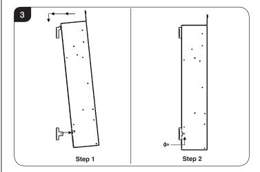
2.23 Use two No. 6 x 12 screws from the kit to fix the fire through both sides into the holes in the lower bar.
