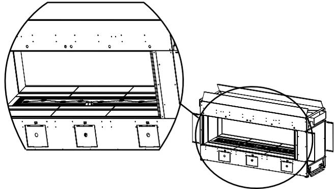
4. Slide in the #4 side panels and secure them by tightening the two screws installed in step 1. Repeat with the #4 side panel on the opposite side.
