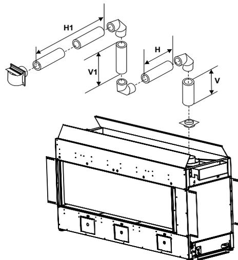
**Venting Arrangement for Vertical Terminations - 5" x 8" (127 mm x 203 mm) Rigid and Flex Pipe (Non Power Vent)**
