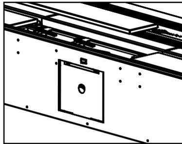
2. From inside the unit, push in the tab to release the access panel at the top.
