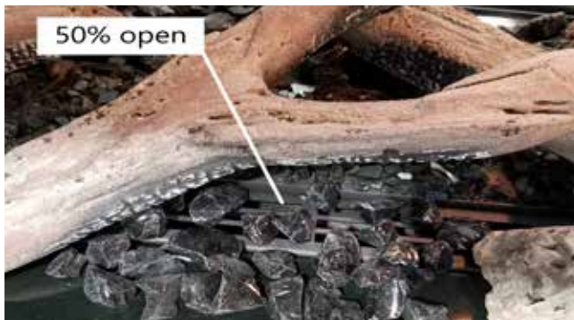
Correct Coal Placement
