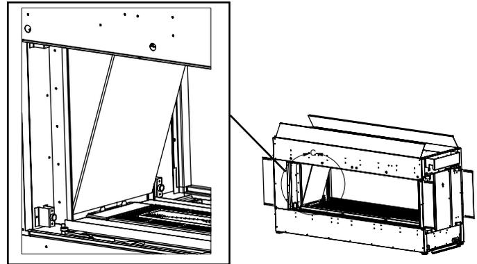
7. Secure side glass by mounting top bracket, then tighten the 2 screws. Repeat steps 5 & 6 on the opposite side.
