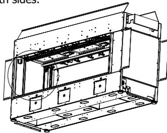
3. Drop the six #3 inner panels into the firebox, then drop the two #2 side covers, as shown below.
