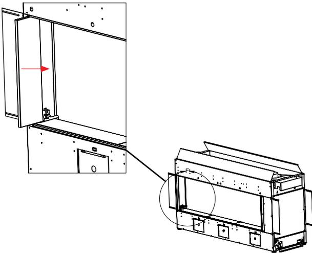
9. Clean the outer panels with a cloth before installing the safety outer barrier glass. To install the safety glass, see this manual for instructions.
