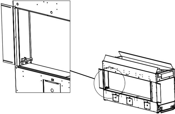
8. Slide the side #5 outer panels between the wall and the barrier stopper bracket. Repeat steps to install the remaining three #5 outer panels using a barrier stop where required.
