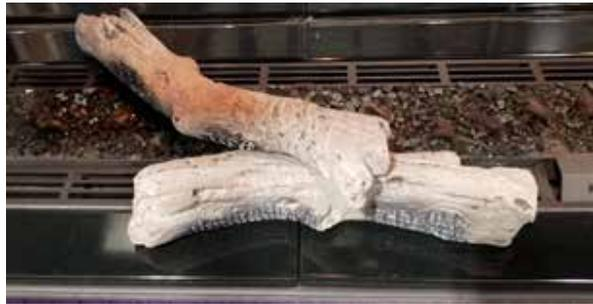
11. Connect the hole underneath Log 4 to the pin on Log 2. Rest Log 4 on the landing on Log 2.
