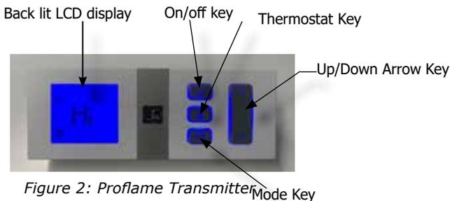
Figure 2: Proflame Transmitter Mode Key
