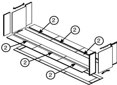
3. Drop the 6 # 2 inner steel panels into firebox. 3 on each side of the burner as per below.
