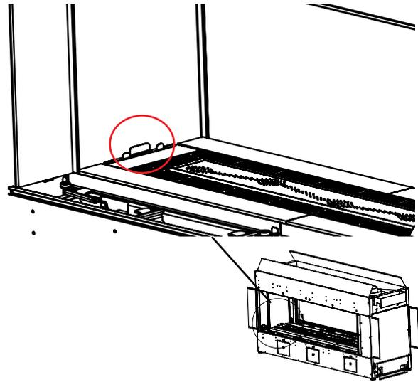
6. Slide the side glass panel #4 into the bottom side bracket.
