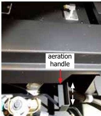
**NOTE** The aeration handle is located near the right side of the gas valve access door, attached by a magnet.
