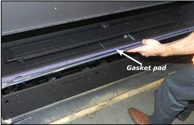
6. Support the glass with one hand and open the 9 lower clamps.
