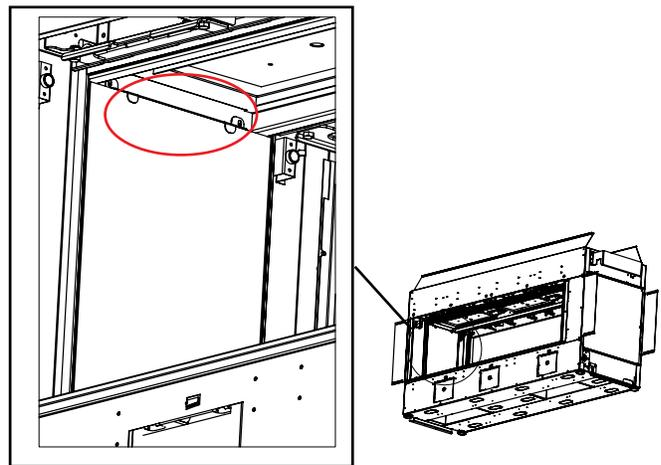
8. Clean the panels with a cloth. Add the desired media or logs before installing the firebox inner glass. To install the firebox glass, see this manual for instructions.
