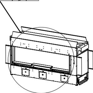
7. Slide the glass barrier stopper in as shown below.
