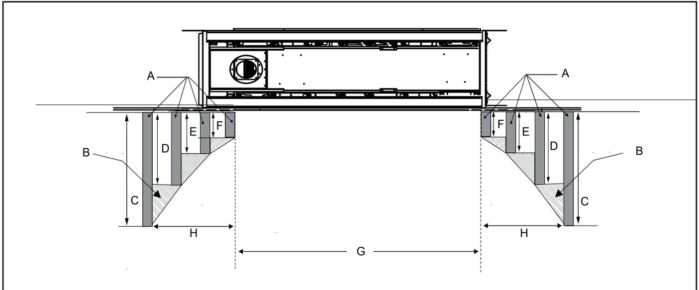
**\*IMPORTANT:** The appliance extends 6-1/16" (156 mm) further on the vent side. See framing dimensions section in this manual for details.
