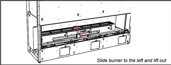
13. Remove burner orifice with a 3/8" wrench. Use another wrench to hold the elbow behind the orifice. Discard the orifice. Reinstall the new burner orifice LPG stamped #50 and tighten.
