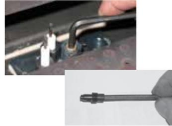
16. Reinstall the pilot cap and pilot retainer clip.
