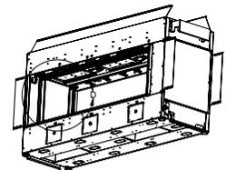
5. Clean panels with a cloth. Add the desired media or logs before installing the inner firebox glass. See this manual for instructions on how to install the firebox glass.
