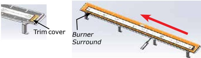
7. Remove eight screws in the locations shown below (four at front and four at rear). Slide the burner to the left, away from the orifice, and lift out.
