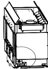
3. Slide electrical box plate towards the back of the unit and then out.
