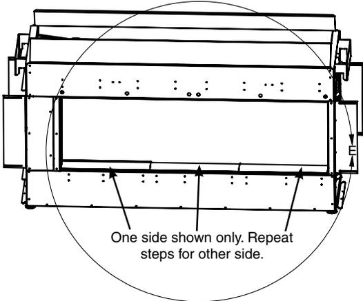
11. Slide the side outer #5 glass panels between the wall and the barrier stopper bracket. If the unit does not have a barrier stopper, stick the side outer panels to the magnets. Repeat steps for the remaining 3 outer sides.
