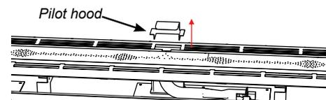
11. Lift off the trim cover on the right side of the burner. Also, remove the burner surround by sliding it to the left and lifting it off.
