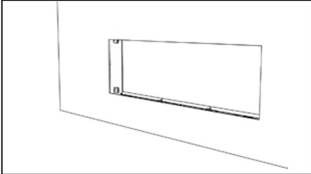
4. Hand bend attachment tabs so they bend past the magnets to the mounting bracket.
