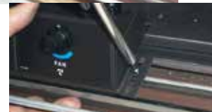
Secure right side with one screw.
