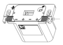
STEP 4 Reinstall wall cover plate with 2 Phillips head screws.
