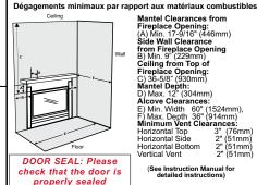
Mantel Clearances from Fireplace Opening: (A) Min. 17-9/16" (446mm) Side Wall Clearance from Fireplace Opening B) Min. 9" (229mm) B) Min. 9' (229mm)
