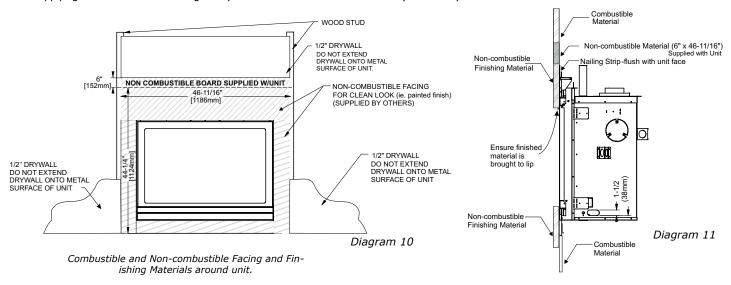
**Note:** The 6" x 46-11/16" non-combustible material supplied with this unit can be replaced if trying to achieve a clean finish. A large piece of non-combustible material (ie. 4' x 8' x 1/2" can be used to eliminate taped seams on or near unit).
