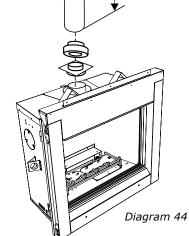
Horizontal Terminations - AstroCap XL & Rigid Rear Vent Kit for Corner Installations - Rigid Pipe 5" x 8"
