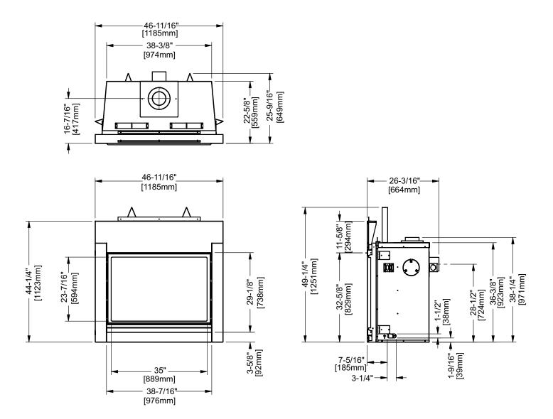
Note: Gas connection is from the right-hand side of the appliance & electrical connection on the left-hand side of the appliance. A metal receptacle box is supplied/installed with the appliance to make all 120 volt electrical connections.
