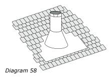
The upper half of the flashing is installed under the roofing material and not nailed down until the chimney is installed. This allows for small adjustments.
