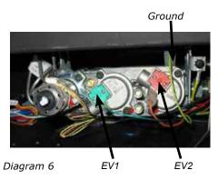
Remove the 14 screws securing the valve tray assembly in place (Diagram and then lift the entire assembly out. Also remove the valve gasket.
