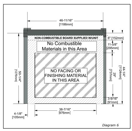
**NOTE:** The 6" x 46-11/16" supplied with the unit is secured directly above the unit as shown above.
