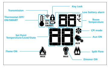
Figure 2: Transmitter LCD Display
