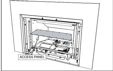
6. The gas flex line can also be disconnected.
