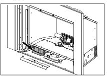
Disconnect the cable coming from the pressure regulator motor at the IFC board (marked X6 on the IFC).
