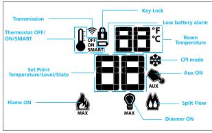
Figure 2: Transmitter LCD Display
