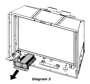
3. Unplug the main power harness (X1) at the PF11 IFC Control Board and disconnect the ground wire from the ground stud.
