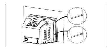
8. Pull the backing plate as far forward as possible against the faceplate, then retighten the screws on both sides.
