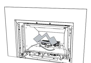
3. Install the rear log #1 and rear brick panel as shown. The rear brick panel is not required as this is optional. Only install the rear brick panel if the optional panel set is being installed.
