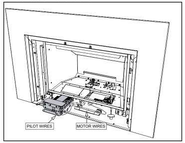
10. Slide the wires through the grommet to remove.
