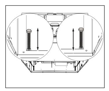
4. The front leveling bolts can be accessed from the front of the insert, on the bottom left and right sides. Once it is in position, adjust the bolts to ensure the appliance is level and won't rock.
