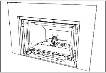
5. Remove the 14 screws securing the Access Panel.
