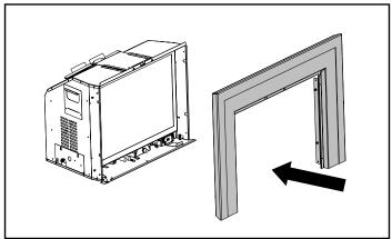
3. Fasten the four screws on both sides to attach the faceplate/finishing trim.
