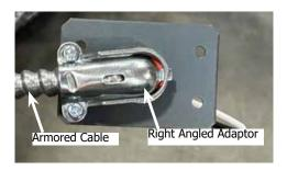
Install bracket onto side cover. Two holes may have to be drilled using a 1/8" bit prior to install, using the bracket as a template.
