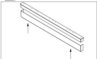
If using a grinder (recommended): trim the lower section to height referring to the installation table for the amount to remove.
