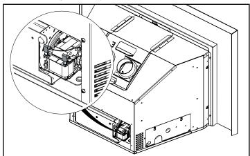
4. Remove fan from unit by lifting up off pins.
