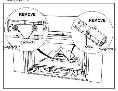
3. Using a Phillips head screwdriver, remove screws securing Rear Deflector.
