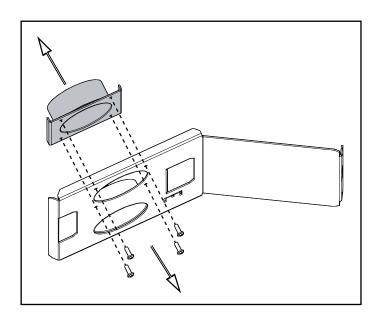
1. Remove the top plate from the unit by undoing the screw at the front of 3. Secure the 2" collar to the top plate using 4 screws in place of the 3" collar.
