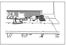
Remove the wire management cover (secured by 2 screws). Remove the wire management straps to access the cables.
