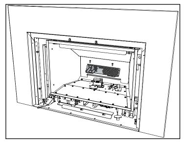
4. Using a Phillips head screwdriver, remove screws securing Pilot Shield.
