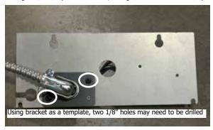
10. Lock the right hand connector using the supplied locking/connector clamp.
