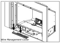
Remove the screw securing the IFC tray and then slid it out to access the motor cable.
