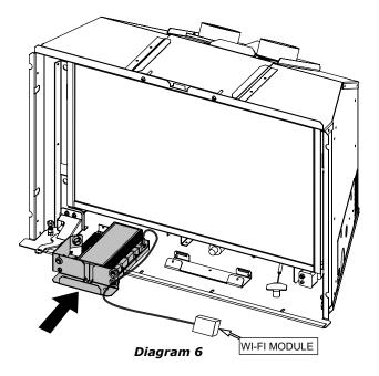
7. Attach the dongle onto the bottom right area of the insert, beside the batteries. The wires can be tucked in with the others under the Wire Cover.
