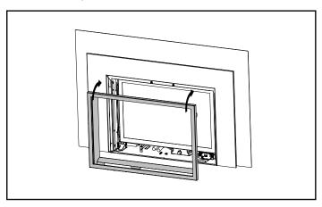
10. Ensure the screen is centered with the faceplate by shifting the screen left or right.
