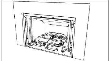
12. Reverse steps 11-1 to replace with new gas valve assembly.
