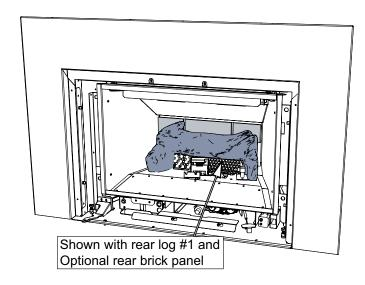
4. Reinstall and secure both the burner and the aeration cap removed in step 2a & 2b. Do not overtighten the aeration cap screw when re-installing. Move the aeration handle to check that it still functions correctly.
