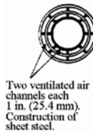
Minimum chimney clearance to sheet steel supports and combustibles 2 in. (50.8 mm)
