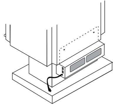
**CAUTION: The connection cord should not be in contact with any hot surfaces. Do not route cord under or in front of unit.**
