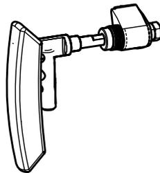
The cool to touch door handle is designed to be inserted from the bottom up and slide off when not held in place. Once in position, the door can be opened. After use, store the door handle on the storage hook located on the left side of the faceplate
