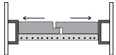
**Note: When getting the chimney cleaned, remove the baffle bricks for access to the flue, then replace them when cleaning is completed.**
