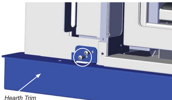
Diagram 3—Hearth Trim Secured to Backing Plate
