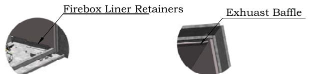
Bottom Right of Firebox
