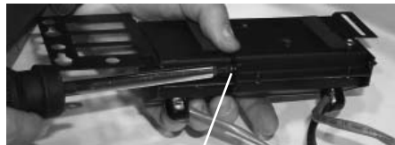
Secure the 2 boxes together with one screw.
