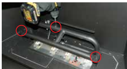
Diagram 2: Slide burner assembly to the right—then remove.
