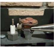
9. Pull off the pilot cap to expose the pilot orifice.
