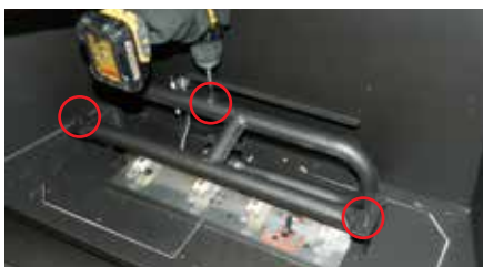
Diagram 2: Slide burner assembly to the right—then remove.
