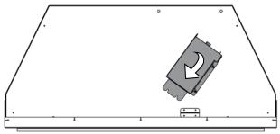
8. Pull the IFC Box to the front of the unit with the two screws showing.
