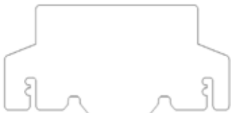
Restrictor plate for Set 1, Set 2 (Part # 761-060F)
