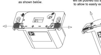
The battery compartment will be pushed out slightly, to allow to easily extract it
