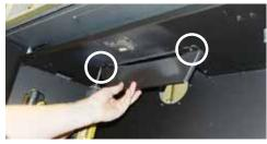
Loosen 2 screws on pilot assembly in locations shown below.
