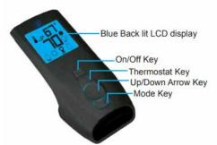
Figure 1: Proflame Transmitter
