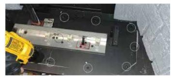
Remove 8 screws from the firebox floor access panel as shown.
