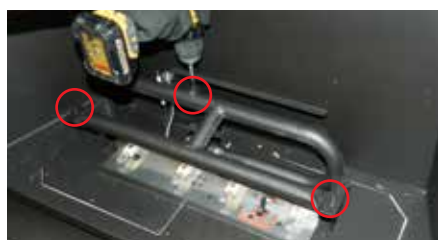
Diagram 2: Slide burner assembly to the right—then remove.
