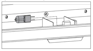
8. Reverse steps to re-install. NOTE: Be careful not to pinch the wiring when re-installing the Top Light Casing. There is a cut-out for the wiring to route through.
