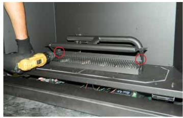
3. Lift up and slide light assembly cover forward to remove.
