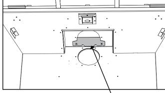
Diagram 2: Vent restrictor located on top exhaust assembly
