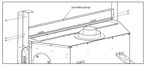
5. Slot the Standoff Deflector onto the back screws, then secure the with a screw through the remaining front hole on each flange.
