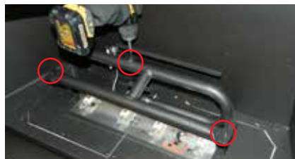
Diagram 2: Slide burner assembly to the right—then remove.
