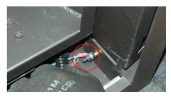
6. Install fan assembly onto pins on unit floor.
