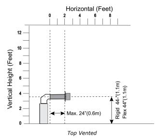
Set #1 (2" open) up to 1' horizontal Factory Setting - no restrictor required greater than 1' horizontal
