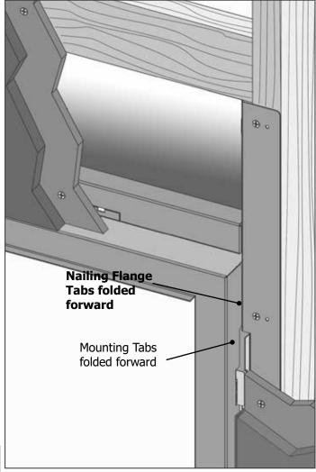
Install the faceplate by resting the arms on the Face Plate on top of the mounting tabs.
