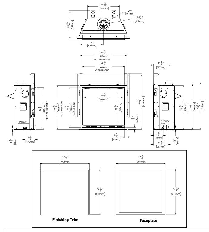
Note: Gas connection is from the left hand side of the appliance & electrical connection on right hand side of the appliance. A metal receptacle box is supplied/installed with the appliance to make all 120 volt electrical connections.
