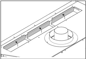
4. Insert a large slotted screwdriver into the slot in between front and back tabs—bend the three (3) tabs up  $90^\circ$  towards the front.
