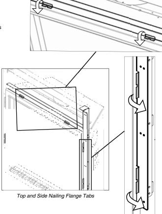
A 1/2" gap must be maintained on the sides and top of the fireplace to allow the finishing trim to be installed and removed. The finishing trim has adjustment for material to protrude up to 1/4" past the front of the finishing trim.
