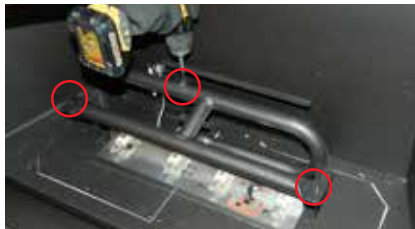
Diagram 2: Slide burner assembly to the right—then remove.
