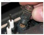
Unscrew the pilot orifice with the Allen key; then replace with the LPG pilot orifice, provided in the kit.
