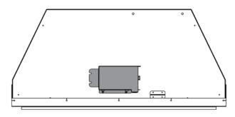
Remove the two screws that secure the Cover Plate to the IFC Mount. Then remove the Cover Plate.
