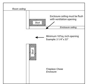
Example 2: Ventilation opening reveal at room ceiling
