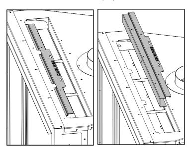
6. Flip top panel 180° and reinstall to top of unit with four(4) screws in locations shown below.
