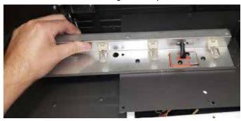
9. Lift out access panel with light assembly and set aside.
