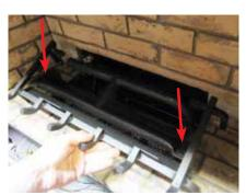
Diagram 1: Remove the left and right screws.
