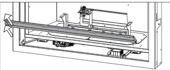
5. Loosen the two Phillips-head screws as shown. They do not need to be removed.
