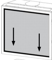
4. Swing screen outwards while keeping the screen level and remove.
