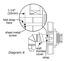
9. Install wall thimble in the center of wood screws the 10" square and attach with wood screws (Diagram 7).
