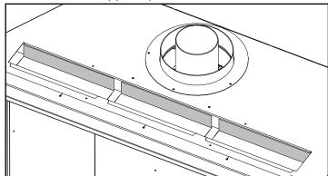
3. Slide out tab as shown to remove—recycle part.
