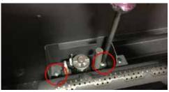
4. Install back panel carefully. Tilt panel forward from the top and rest the bottom of the panel on the firebox floor. Tip top back until it also rests on the firebox back wall.
