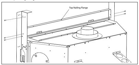
Slot the Standoff Deflector onto the back screws, then secure the with a screw through the remaining front hole on each flange.
