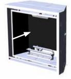
9. Slide the bottom panel carefully underneath the burner and push to the back until it contacts the back panel.
