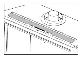
5 . Bend the rear three (3) tabs up  $90\ensuremath{^{\circ}}$  towards the back of the unit.
