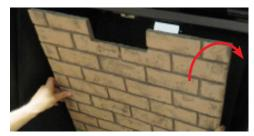
5. Loosen screws and remove brick clip.
