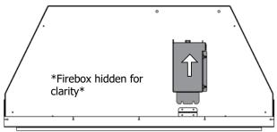
7. Rotate the front of the IFC Box to the left.
