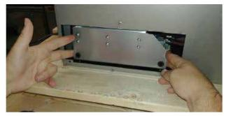
Secure fan access panel back onto the unit with 4 screws (locations shown below).
