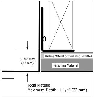
(Outside Finish Only) A 1/2''(13 mm) gap must be maintained on the sides of the fireplace to allow the Faceplate to be installed and removed. See Faceplate Finishing in this manual for guidelines if you're installing the optional faceplate.
