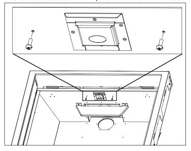
5. Remove the Top Light Casing by lifting up and out.
