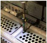
Add 7 lbs of crystal media and spread it across the tray in one even layer. Important: ensure that at least 50% of the gas burner porting remains uncovered. Do not cover the pilot area.
