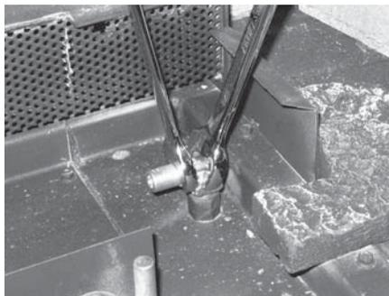
Burner Orifice Removal
