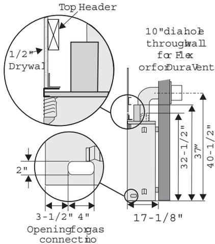
**Note:** 40-1/2" (1029mm) is the minimum height for both flex termination or Simpson Dura-Vent venting.
