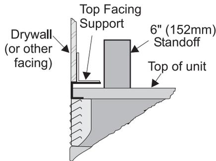
Install Side Nailing Strips, Top Facing Support, and Top Standoffs before unit is slipped into position. See page 9 for assembly details.
