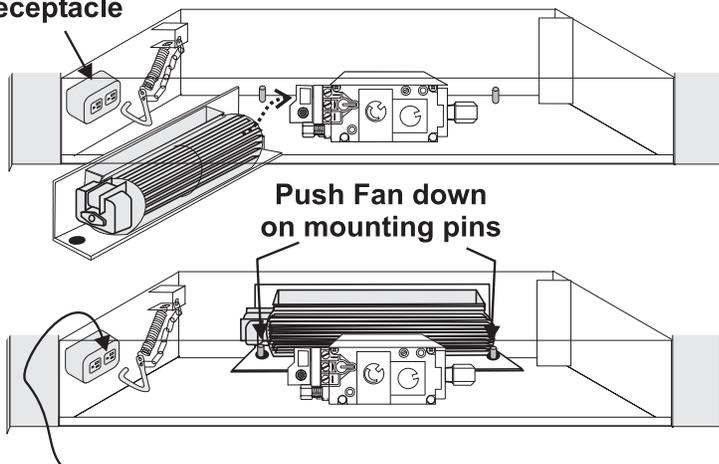
Plug fan power cord into rear receptacle.
