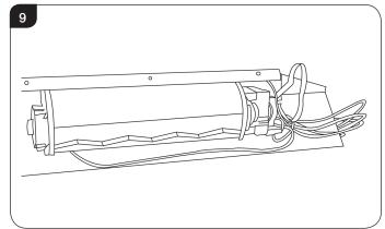
8.7 Replace in reverse order ensuring the wires are put back in exactly the same configuration.
