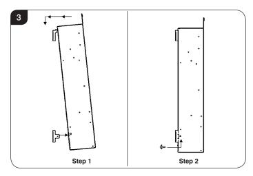
2.23 Use two No. 6 x 12 screws from the kit to fix the fire through both sides into the holes in the lower bar.
