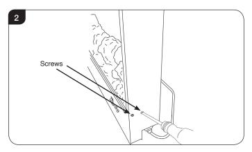
4.3 Remove the 4 screws on the back (2 on either side of the back), see Diagram 3.
