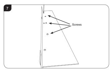
8.5 Remove the 3 screws at the top of the back of the appliance.
