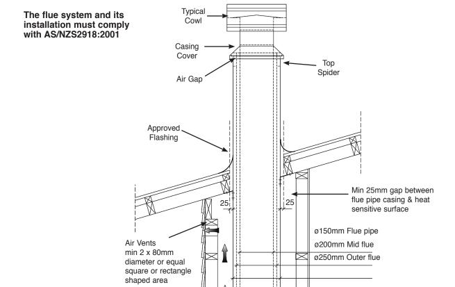
Note: All external air vents & ceiling penetrations must be bird & rodent proofed with permanently fixed screens
