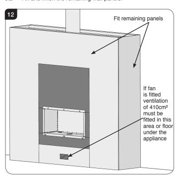
If a convection fan is to be fitted, leave a convection hole in the lower panel below the front of the opening. This hole must have a minimum free area of 410cm<sup>2</sup>.
