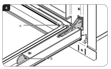
5b.3 Open and close the door a few times to work the grease into the hinge to return it to smooth operation.
