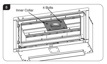
5d.2 The 2 x longer front bolts are recessed into the collar, see Diagram 9.
