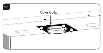
11.7 There is a Flue Collar Bracket on top of the Outer Box. This locates on two pins that allow flexibility when replacing the Outer Collar. The bracket remain in place when installing the flue system, see Diagram 18.
