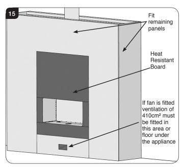
9.6 Apply a heat resistant plaster finish to at least 900mm above and 400mm to the sides of the chimney breast, making sure it is not too thin or it will crack, see Diagram 16.
