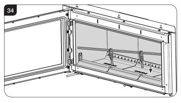
Slide the Log Guard across so both end locate evenly in the holes in the side bricks, See Diagram 35.
