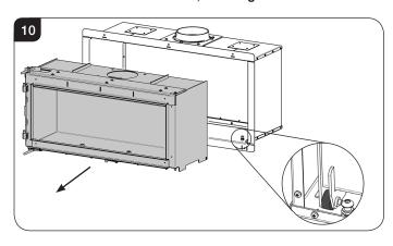
Pull the inner box carefully forward to release from the cutouts. It should now slide smoothly out of the outer box.
