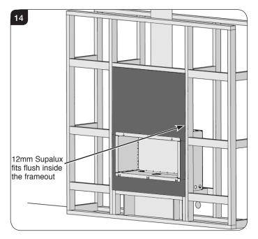
9.5 Fit another layer of Heat Resistant Board to the highlighted area ensuring it is at least 400mm to the sides and 900mm above the appliance.
