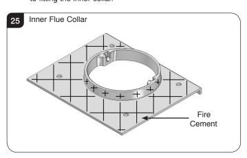
13.3 Fit the inner flue collar using the 4 x bolts ensuring the top hat spacers are replaced on the 2 x longer front bolts, see Diagram 26 and all bolts are finger tight only.
