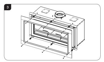
3.5 Secure the frame to the appliance body using the screws and nuts provided, see Diagram 4.
