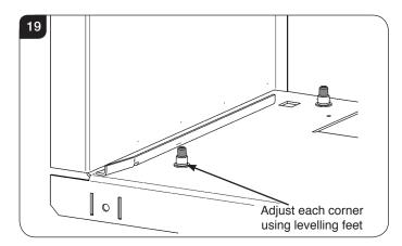
11.11 Wind the set screws down to the desired position in each corner.
