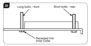
13.4 Ensure that the front of the inner box is parallel to the outer box, see Diagram 27. Adjust the position until correct and then fully tighten the 4 x bolts. Do not over tighten.
