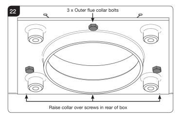
12.2 To ensure the outer collar is central, and **to avoid cross threading of the bolts** during actual installation, feed the 4 x bolts used to secure the inner collar into the holes in the outer collar as shown in Diagram 23. This should be done by hand and the bolts should be finger tight only. Do not force the bolts. If they are not easily located remove them and loosen the 3 x bolts holding the outer collar to allow for adjustment.
