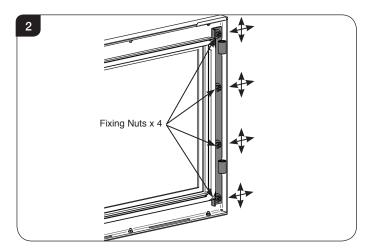
5a.5 Loosening the Door Hinge Assembly allows for fine vertical and horizontal adjustment of the door position. This may require a trial and error approach to find the correct position. Ensure the door is horizontal before tightening the fixing nuts.
