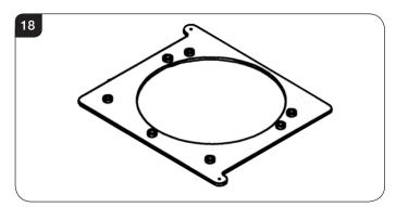
11.8 If the optional fan is to be fitted, remove the fan cover in the base of the outer case. This cannot be removed after the outer case has been installed. Full instructions are included with the fan (PM379).
