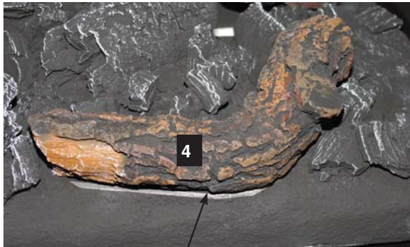
Ridge in burner tray (highlighted)
