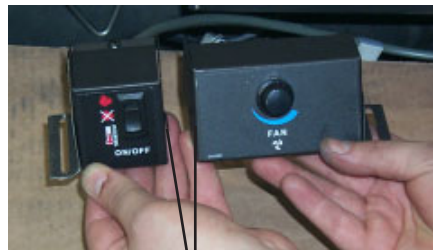
Diagram 3: Use the clip & hook on the side of the control boxes to join them together.
