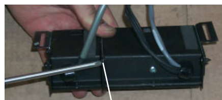
Secure the 2 boxes together with one screw.
