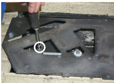
Diagram 1: Remove the left screw and then slide the burner assembly away from the orifice and lift out.
