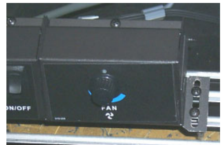
Secure right side with 2 screws.
