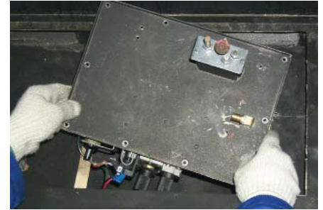
Lift entire valve tray assembly out.
