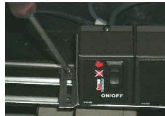
Secure left side with 2 screws.
