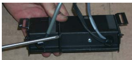
Secure the 2 boxes together with one screw.
