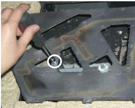
Remove the screw on the left side of the burner.
