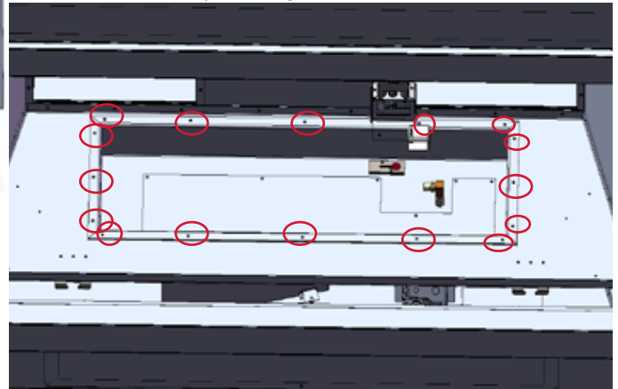
Diagram 4 - Valve Tray Screw Locations
