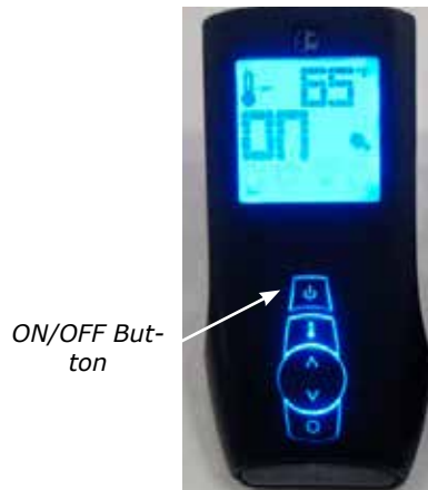
Diagram 1 Remote shown in Manual Mode on Hi
