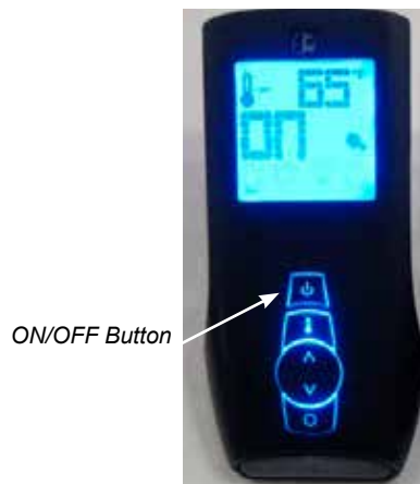
Diagram 1 Remote shown in Manual Mode on Hi
