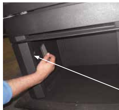
Handle stored on hanger in wood storage area.
