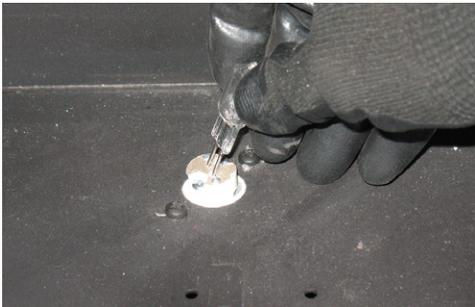
14) Install two light diffusers on to the base tray.
