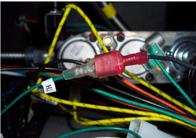
4. Connect the other thermostat lead to male connector disconnected from Step 1 using a female spade connector - see picture below.
