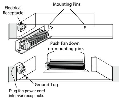
8. Connect and secure fan ground cable to ground lug.
