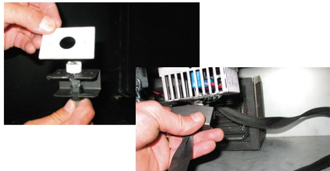
12) Install each light assembly from the underside of the floor of the firebox. Secure with 2 screws as shown below.
