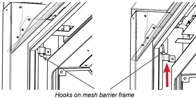
2. When hooks are clear of the bracket—tilt mesh frame out slightly from the bottom and manoeuvre mesh out.
