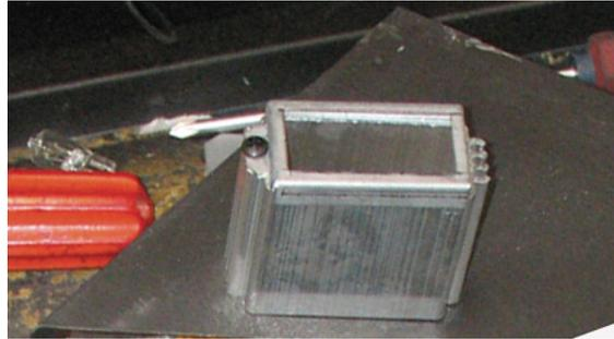
15) Secure diffusers onto base tray from the backside of the tray with 2 screws.
