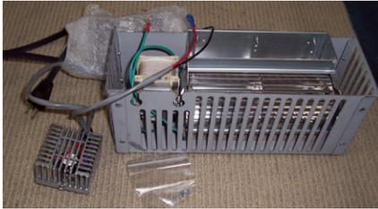
4. Connect the **Black** wire to the left side terminal of the fan motor. Slide the black wire and the green ground wire into grommet and push grommet into the fan assembly housing.
