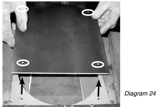
**Before proceeding to Step 8,** inspect condition of all gaskets. DO NOT install parts with damaged gaskets. Replace if necessary with spare gaskets supplied.
