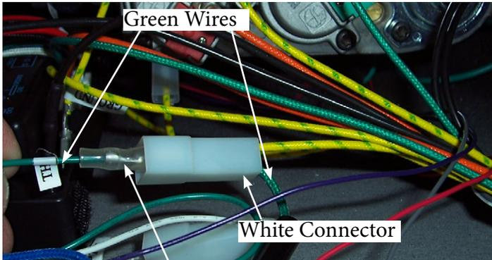
3. Connect one thermostat lead to female connector, using male spade connector - see picture below.
