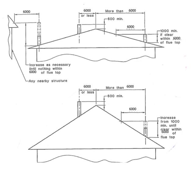
THE FLUE PIPE SHALL EXTEND NOT LESS THAN 4.6 M ABOVE THE TOP OF THE FLOOR PROTECTOR. NOTE: INSTALLATION MUST BE CARRIED OUT BY A LICENSED INSTALLER IN ACCORDANCE WITH AS/NZS 2918:2001
