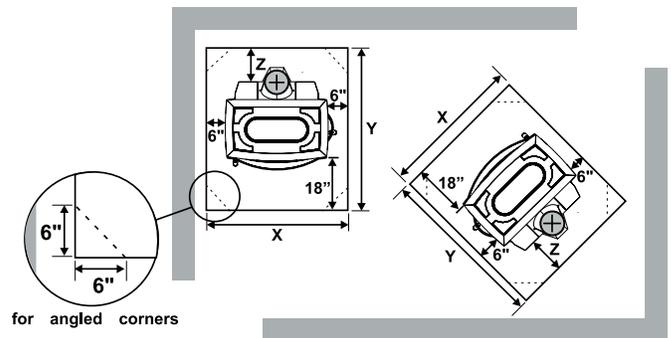
**NOTE: In Canada, floor protection must extend 18" to the front and 8" to each side of the stove.**
