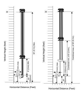
The shaded area in the diagrams show the allowable vertical terminations.
