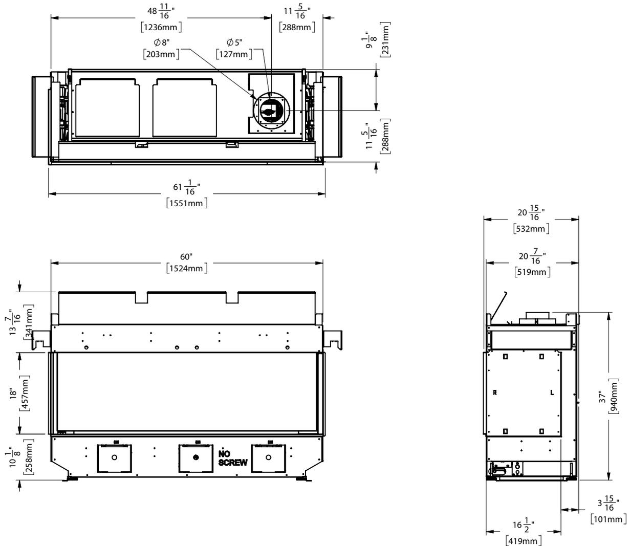
**Note:** Height Dimension is taken with leveling legs fully inserted and may vary depending on the height of the leveling legs, when unscrewed or extended.
