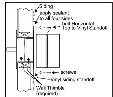
The four wood screws provided should be replaced with appropriate fasteners for stucco, brick, concrete, or other types of sidings.
