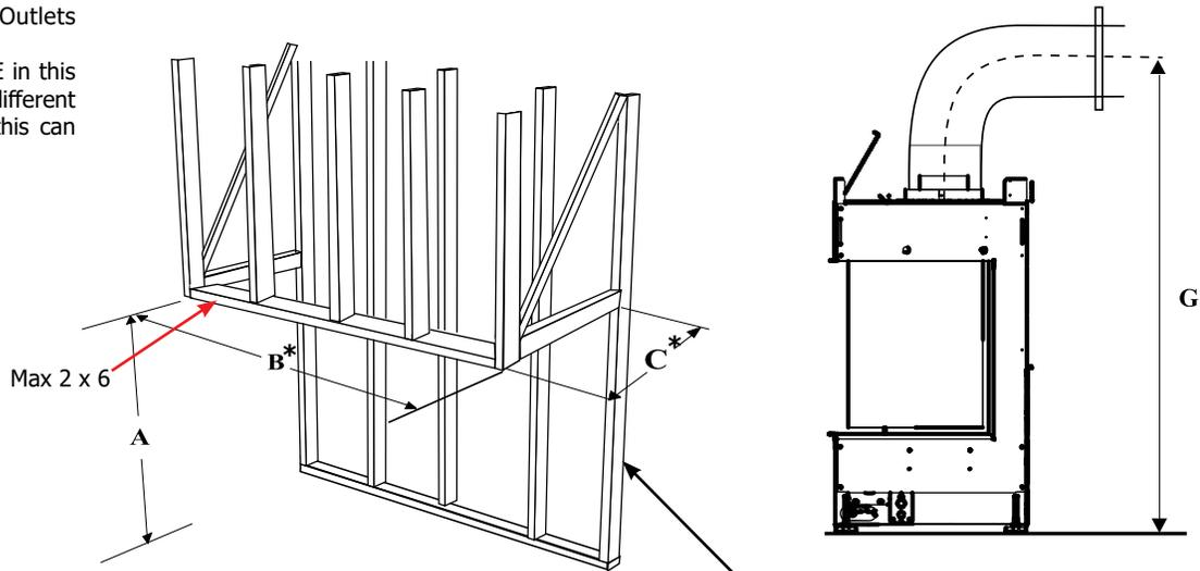
Note: This appliance must be installed on a solid surface such as a plywood floor which must be the full width and depth of the appliance.
