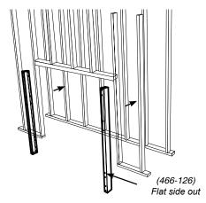
Secure horizontal steel header stud (466-128) with 2 screws per side as per diagram.
