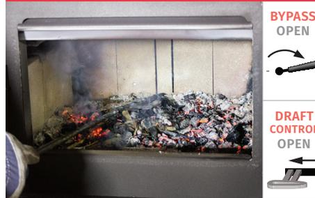
1) With the unit and chimney now up to operational temperature the reloading process will require less time. At the end of the burn cycle and to restart the unit, turn off the fan before opening the door and **spread the coals out with a poker**.
