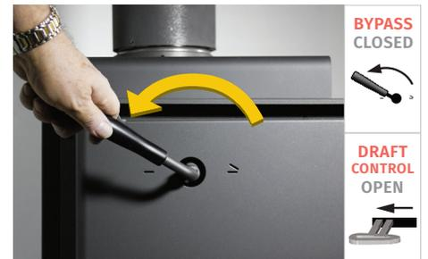
4) Once the fire becomes established add large logs to the firebox until it is fully loaded. Typically, after 20-30 minutes you should be able to **close the bypass damper** as temperatures will have reached the "active" zone (beyond 500°F, 260°C).
