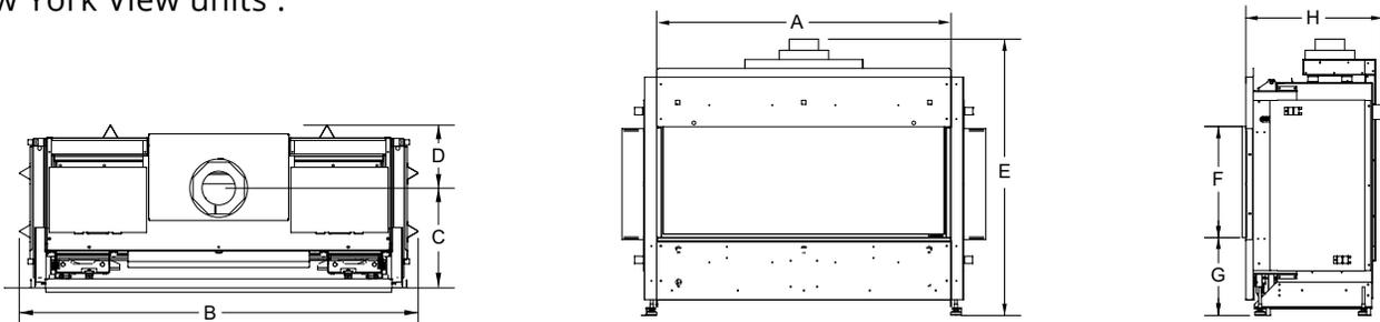
NOTE: CV50E flue is on the side
