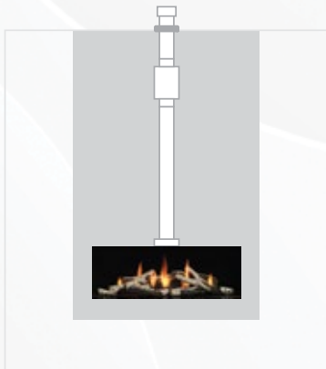
Inline Power Vent system shown vertical vent run
