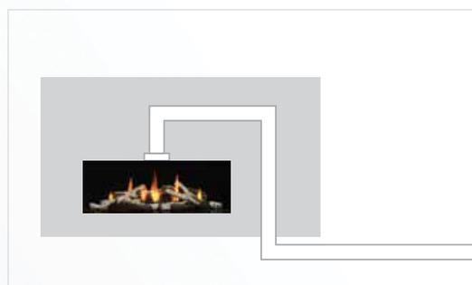
End of line flush horizontal Power Vent
