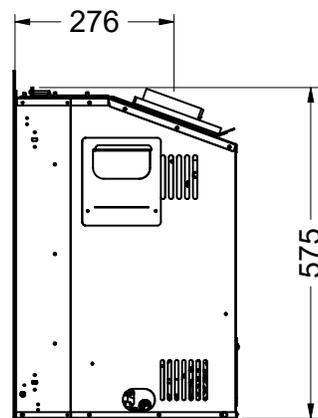
**Unit Dimensions - With Backing Plate (millimeters)**
