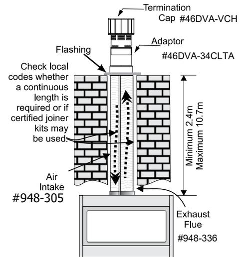
Note: When installing the flueing, identify the flues. Mark one exhaust and one intake as indicated on the top of the unit.
