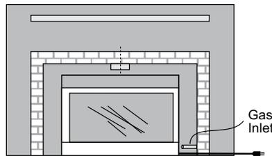
NOTE: Shut off valve must be installed in an accessible location.
