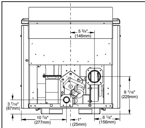
Insert Inlet and Outlet Location
