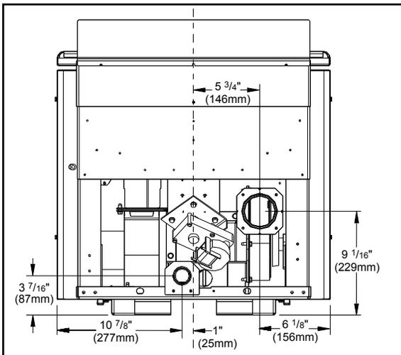
Insert Inlet and Outlet Location
