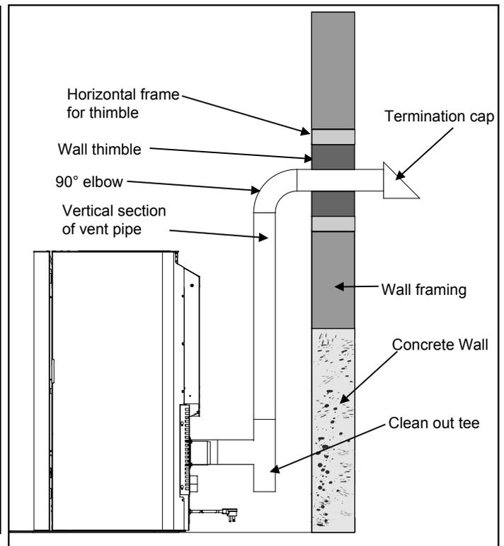
Figure 2 - Venting with Concrete Wall Behind Unit
