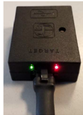
Fig.3: WiFi dongle connected to the IFC
