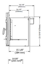
NOTE: Before assembling your Insert, use these dimensions to ensure appropriate clearances will be met (refer to Masonryand Factory Built Fireplace Clearances section).
