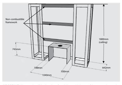
IMPORTANT: Non-combustible sheeting of a minimum thickness of 9mm must be used on the front face of the enclosure.
