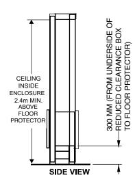
${\tt NOTE:} Enclosure\ depth\ will\ depend\ on\ the\ the\ finished\ wall\ thickness\ on\ each\ side\ of\ the\ enclosure\ -\ see\ installation\ manual\ for\ details.$
