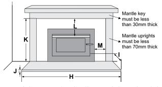
Note: Hearth clearances can be reduced by raising the heater above the hearth. Note: Distance "M" & "L" must be non combustible facing
