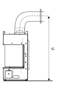
Note: This appliance must be installed on a level and solid surface such as a plywood floor which must be the full width and depth of the appliance.
