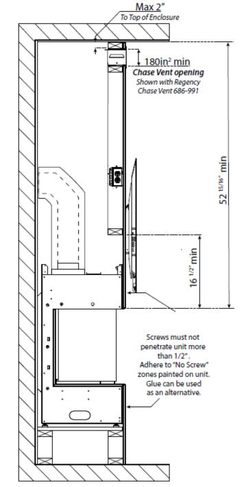
Note: The TV mounting bracket cannot be secured directly to the appliance. It must be secured to framing. The TV depicted in the picture may need to be higher depending on the style of TV mounting bracket used.
