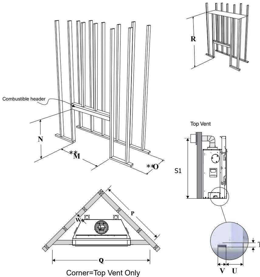
\*\*The framing depth/width does not take into account dry wall/wood or similar materials against the back /side wall. The framing depth will need to change based on the thickness of the material
