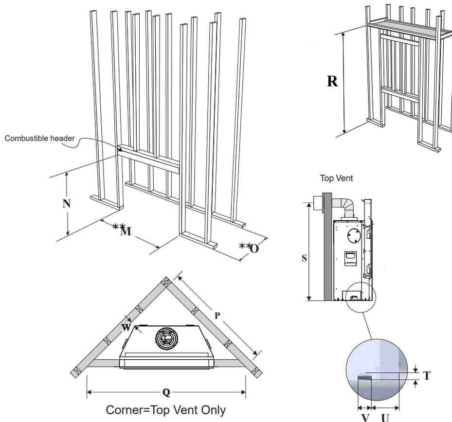
\*\*The framing depth/width does not take into account dry wall/wood or similar materials against the back /side wall. The framing depth will need to change based on the thickness of the material
