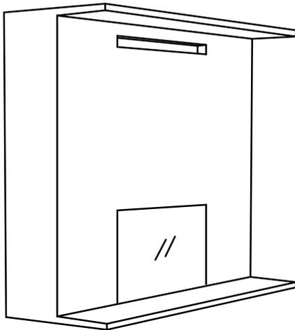
Example 2: Ventilation opening reveal at room ceiling
